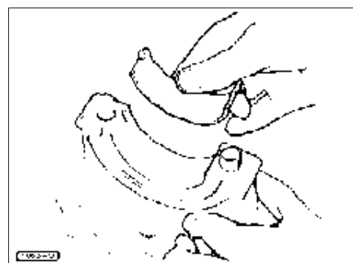
Fig. 20 - Fitting the one main bearing shell into the main bearing cap.
