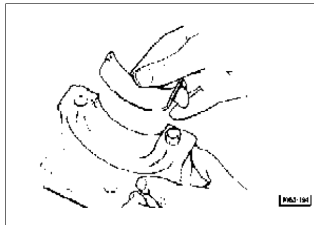
Fig. 20 - Install the main bearing shells in the front and rear crankshaft bearings. Shoulder half rings shall be secured in the rear bearing after applying some grease;
