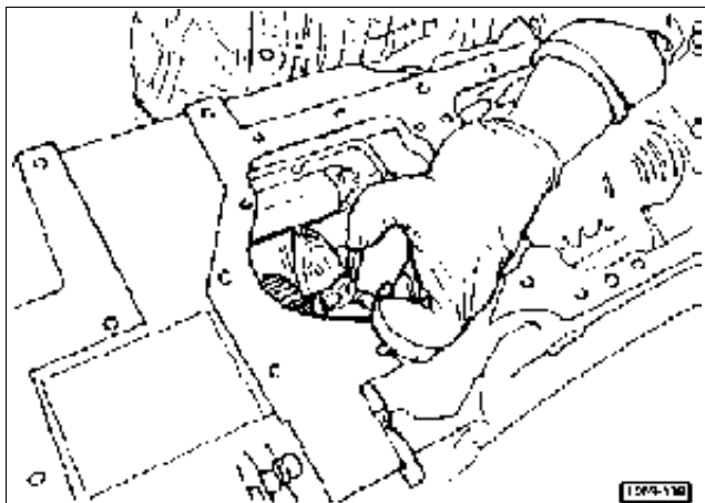
Fig. 25 - Locate the stop circlip on the input shaft of the P.T.O. clutch assembly.
