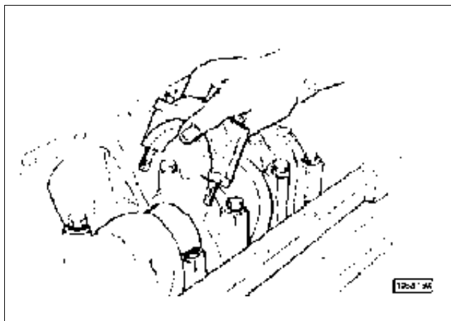
Fig. 19 - Install the intermediate crankshaft main bearing taking care the numbers stamped on the bearing correspond to those stamped on the crankcase. (Numbers should all be oriented in the same direction);
