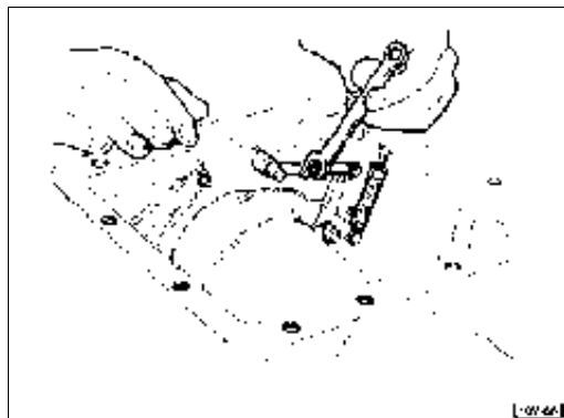
Fig. 13 - Adjusting lifting lever regulating tie rod (yellow).
